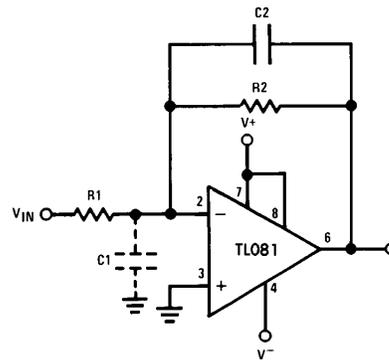
Parasitic input capacitance  $C_1 \approx (3 \text{ pF for TL081 plus any additional layout capacitance})$  interacts with feedback elements and creates undesirable high frequency pole. To compensate, add  $C_2$  such that  $R_2 C_2 \approx R_1 C_1$ .
